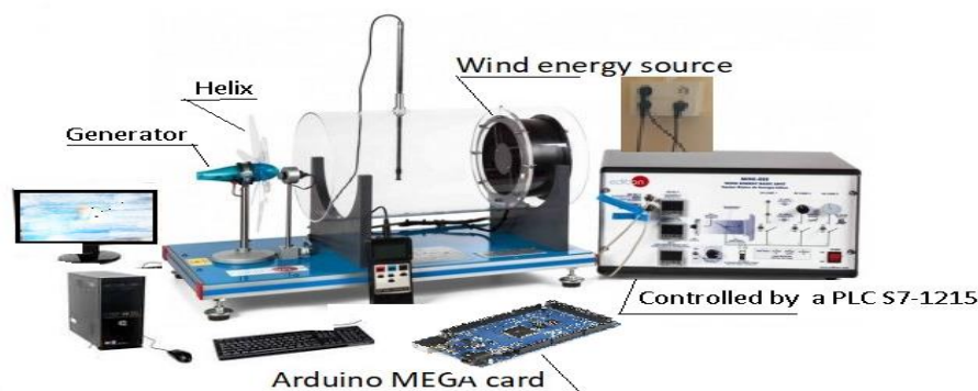
Figure 5. Photography of the experimental bench
