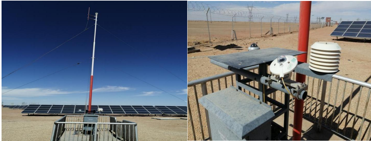
Figure 6. Photograph of meteorological NARI weather station.
