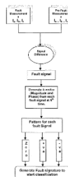
Figure . 2 Logical representation of the use of symmetrical structures to produce fault signs
