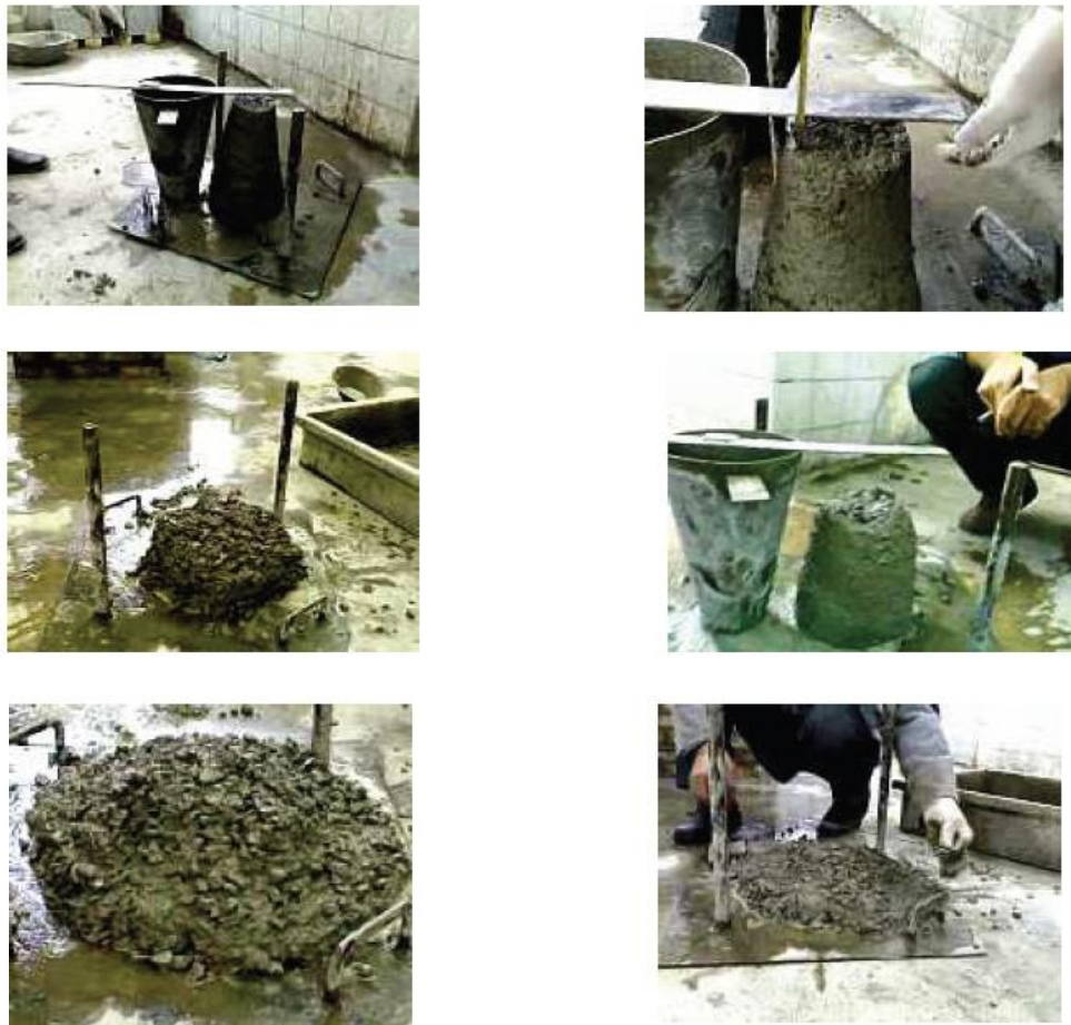
Figure 2. Slump types of concrete mixes
